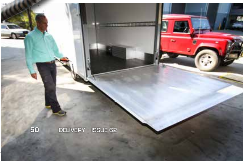
The cityBOX offers a low floor with a shallow angle ramp and power tailgate opening and closure.
