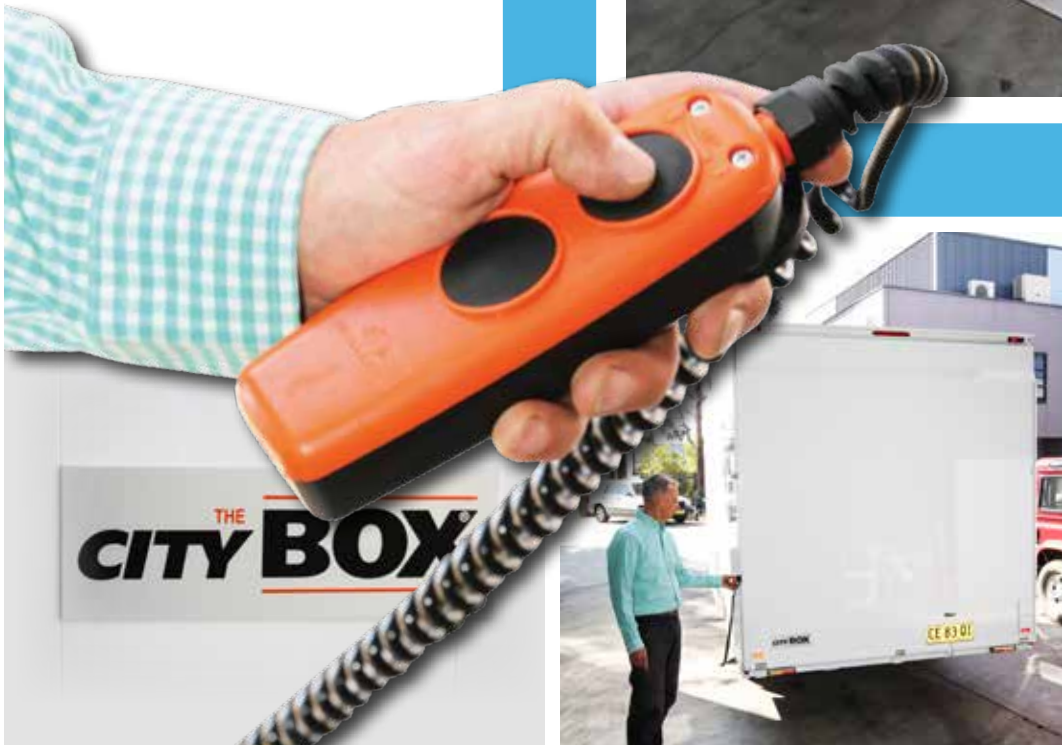
The cityBOX offers a low floor with a shallow angle ramp and power tailgate opening and closure.
